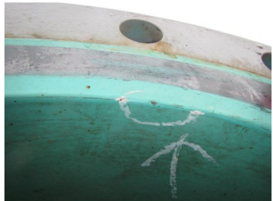
MANWAY NOZZLE COATING FAILURE
