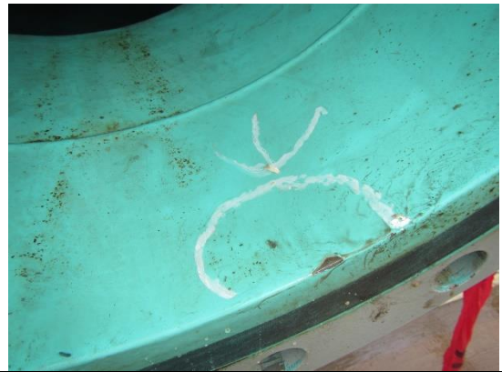
MANWAY NOZZLE COATING FAILURE
