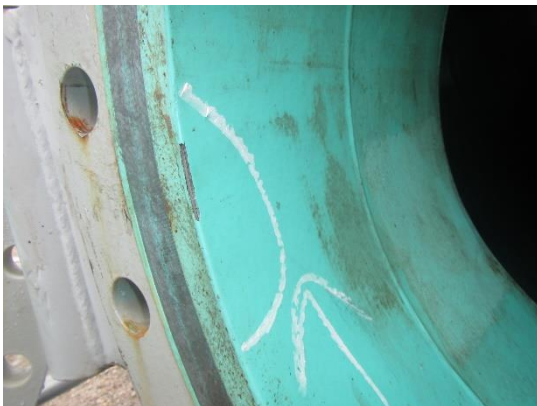
MANWAY NOZZLE COATING FAILURE
