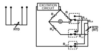
This system provides precision measurements. By switching the pairs of leads and averaging, you arrive at a value from which the lead resistance, thermal emf's in the leads and resistance changes in the leads due to ambient variation has been eliminated.
