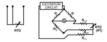
Industrial sensors commonly use this three wire connection system. For this system to be effective, all the leads (R<sub>LA</sub>, B, C) should be very near the same length and of the same gauge.
