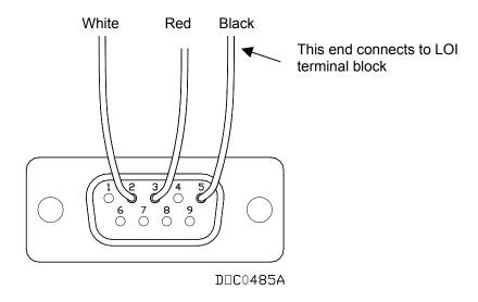
Figure 4-1. Operator Interface Wiring
