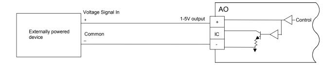
Figure 6-4. 1-5 Volts Analog Output Voltage Control
