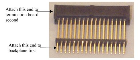
Figure 8-2 . 34-Pin Interface Connector
