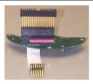
Figure 8-1 . Backplane with 34-Pin Interface Connector
