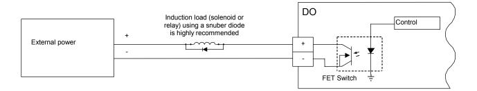
Figure 6-6. Solid State Relays – Discrete Outputs
