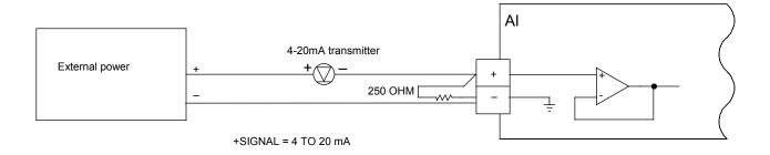
Figure 6-1. Current Signal on Analog Input
