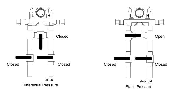
Figure 7-3. Pressure Calibration Open/Close Orientation
