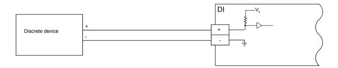
Figure 6-5. Discrete Input Wiring
