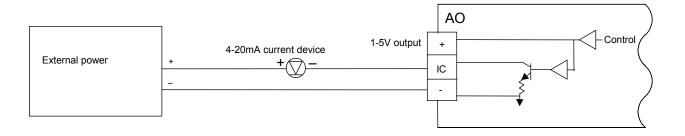
Figure 6-3. 4-20 mA Analog Output Current Control
