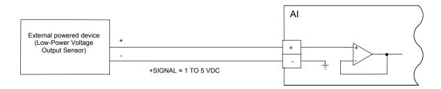
Figure 6-2. Voltage Signal on Analog Input
