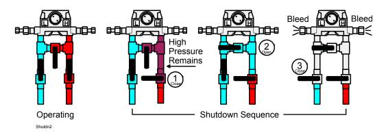
Figure 7-2. Removing the DVS from Service
