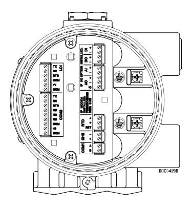
Figure 1-3. Wiring Terminals
