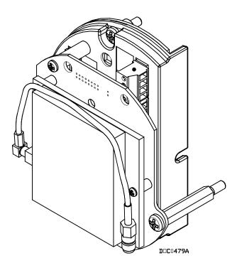
Figure 4-2. Radio and Interface Card (FreeWave shown)
