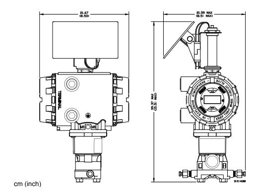
Figure 2-2. Outline and Mounting Dimensions with Solar Panel and LCD
