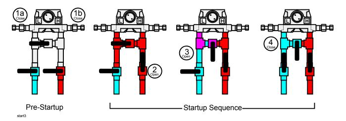
Figure 7-9. Returning the DVS to Service
