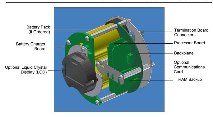
Figure 1-2. Inside the FloBoss 103 Enclosure
