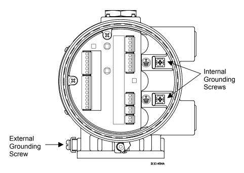
Figure 3-1. Location of Grounding Screws
