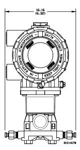
Figure 2-1. Outline and Mounting Dimensions without Solar Panel
