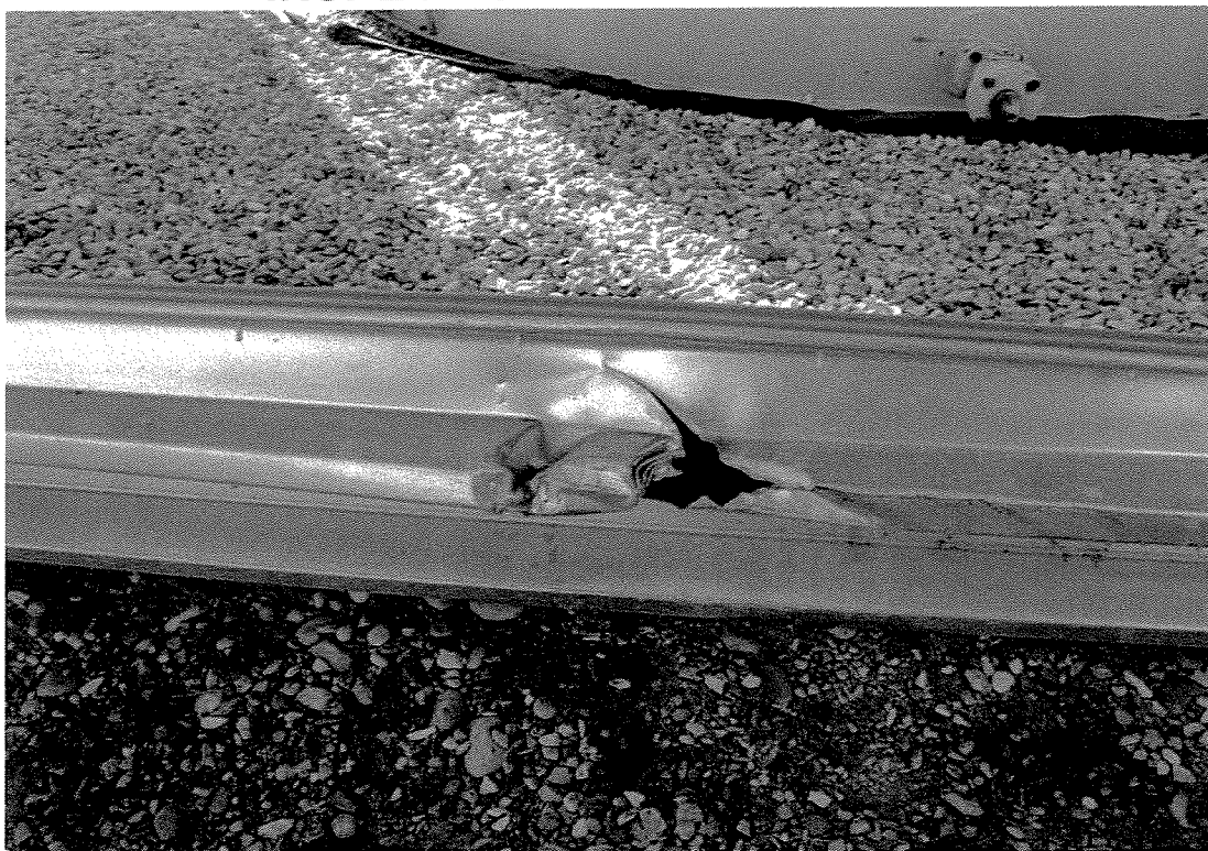
Photo #5: Closeup of containment damage
