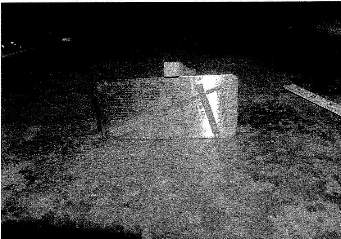
Photo #8: Pit gauge showing 0.050" pitting
