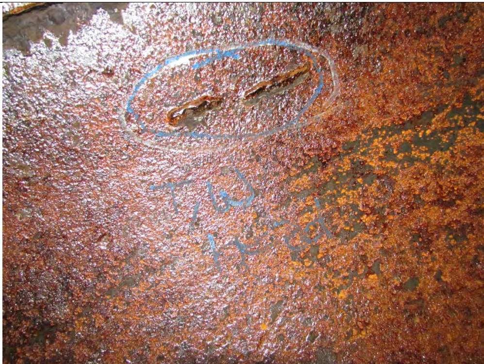
Broken tack weld in top of west head
