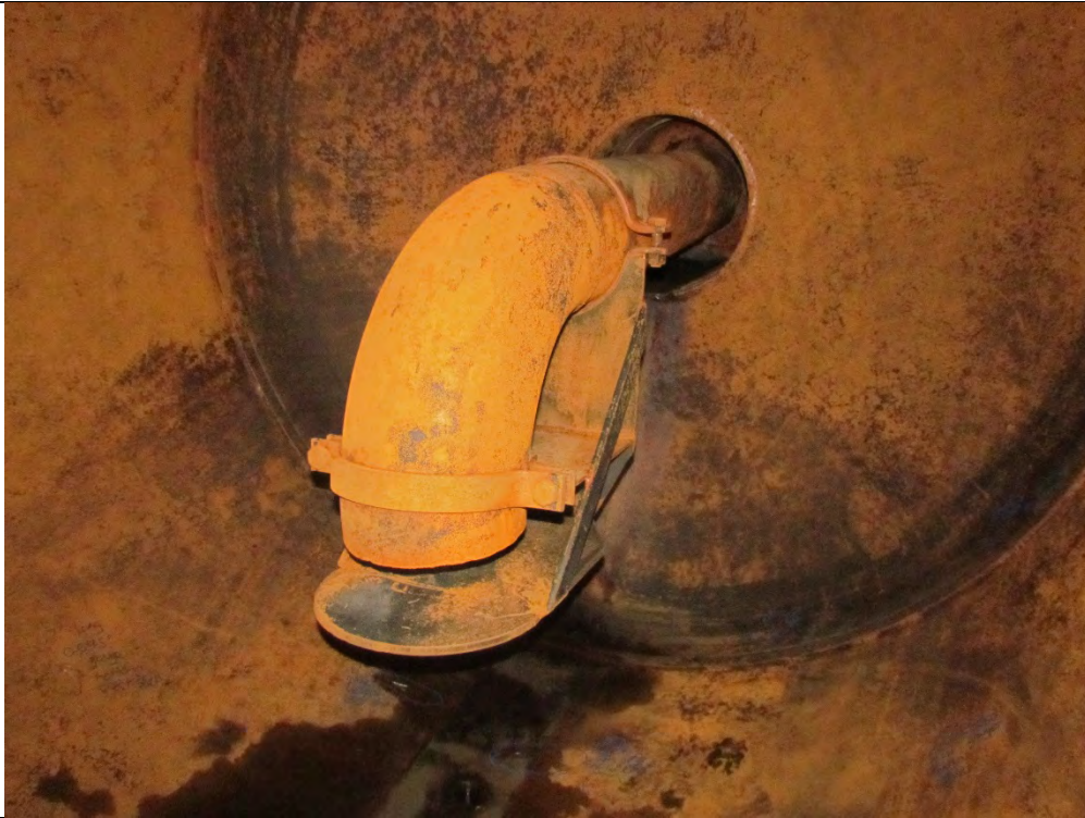
Vessel inlet piping and deflector plate assembly
