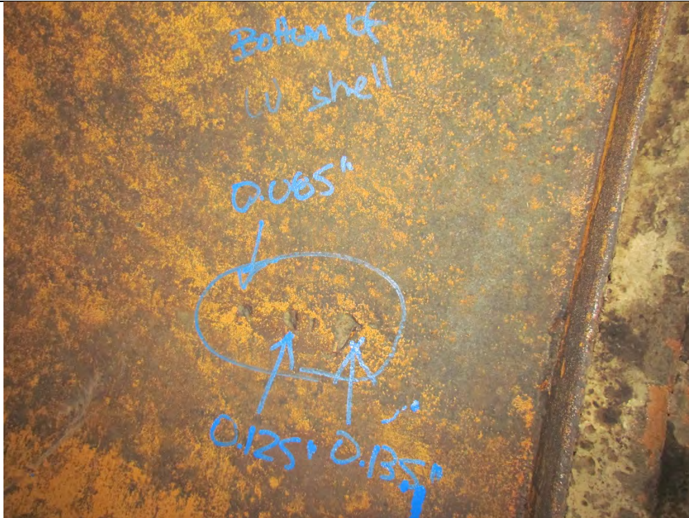
0.065"/0.125"/0.135" defects in bottom of west end of shell
