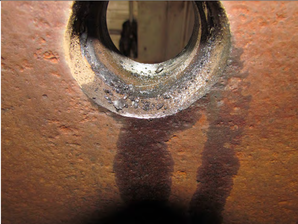
Non full penetration weld for new nozzle
