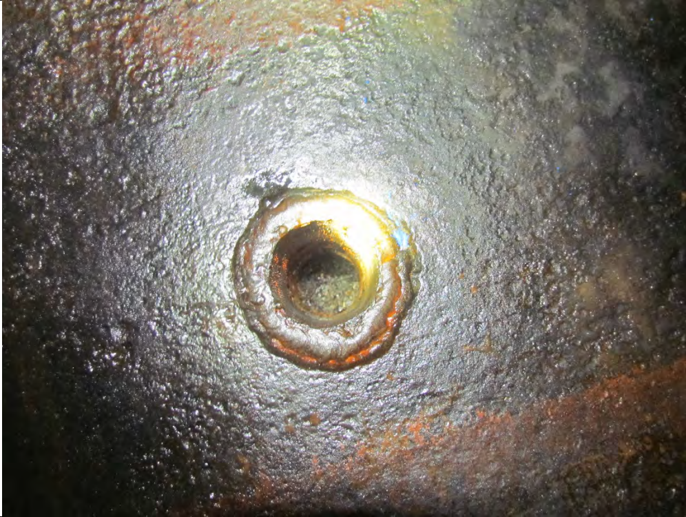
Bottom nozzles were obstructed with debris
