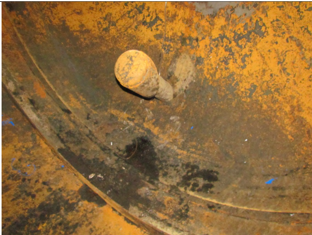
Internal vessel pipe and stiffening ring at west head
