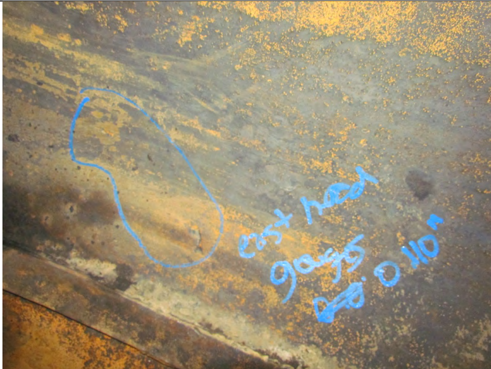
0.110" Depth gouge in east head (bottom)
