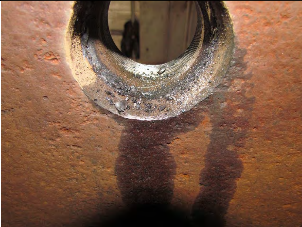
Non full penetration weld for new nozzle
