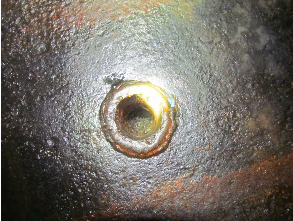
Bottom nozzles were obstructed with debris
