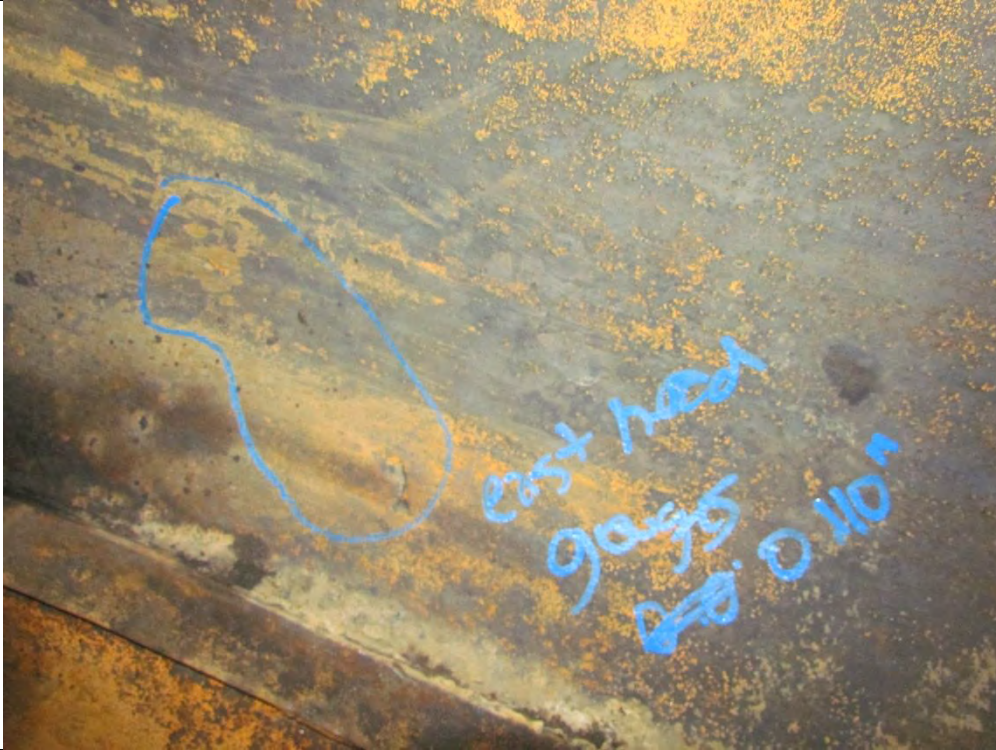
0.110" Depth gouge in east head (bottom)
