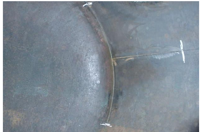
SHELL TO HEAD WELD
