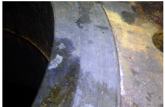
20" MANWAY FLANGE SEALING SURFACE
