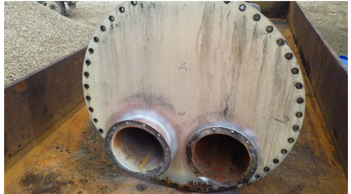
Tube Sheet Overview (Atmosphere side)
