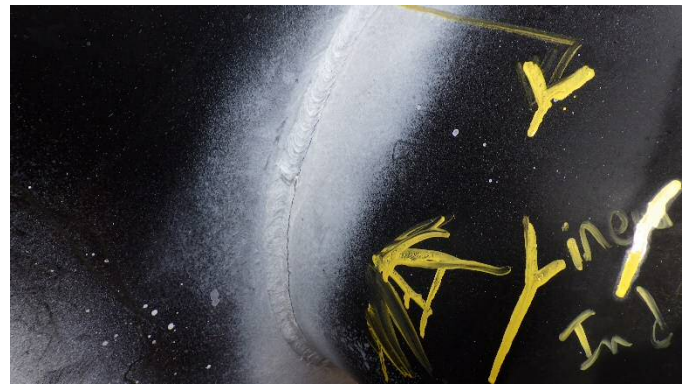
Linear Indication, Exhaust Tube Side
