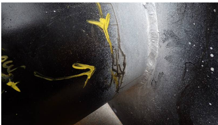
Linear Indication, Burner Tube Side
