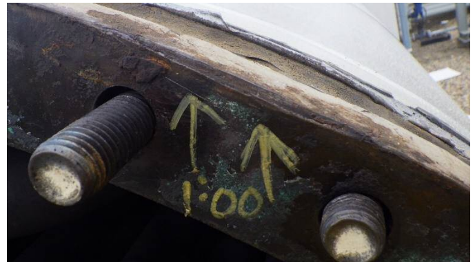
Mechanical damage on west flange Reboiler)
