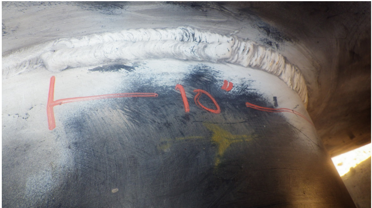
Exhaust side – partial crack #2
