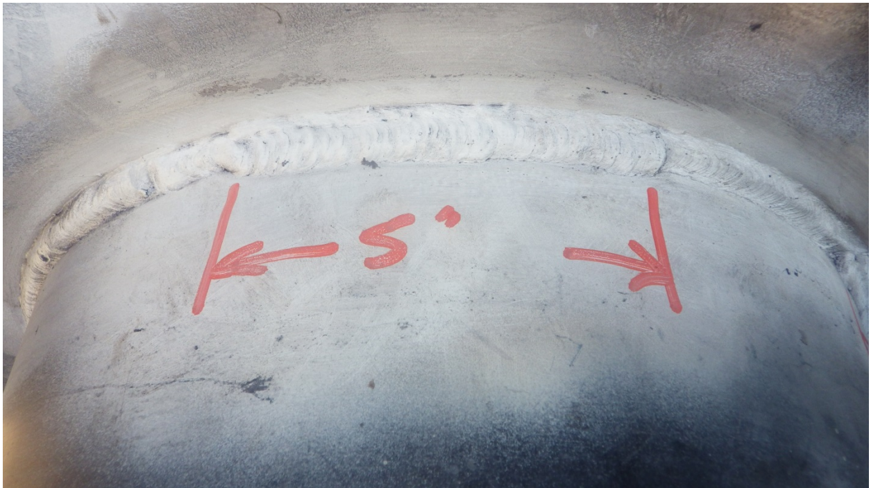
Exhaust side – partial crack #1
