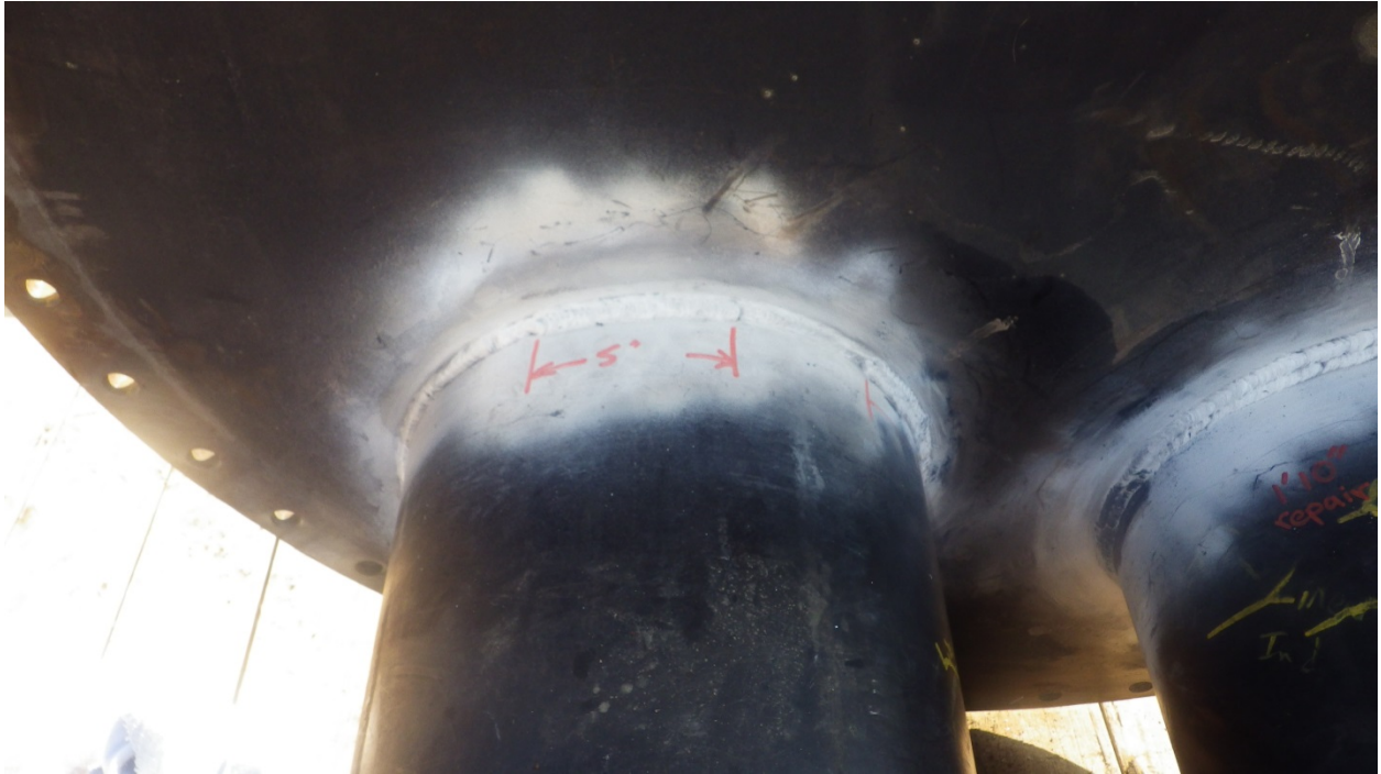
Exhaust side – partial crack #1
