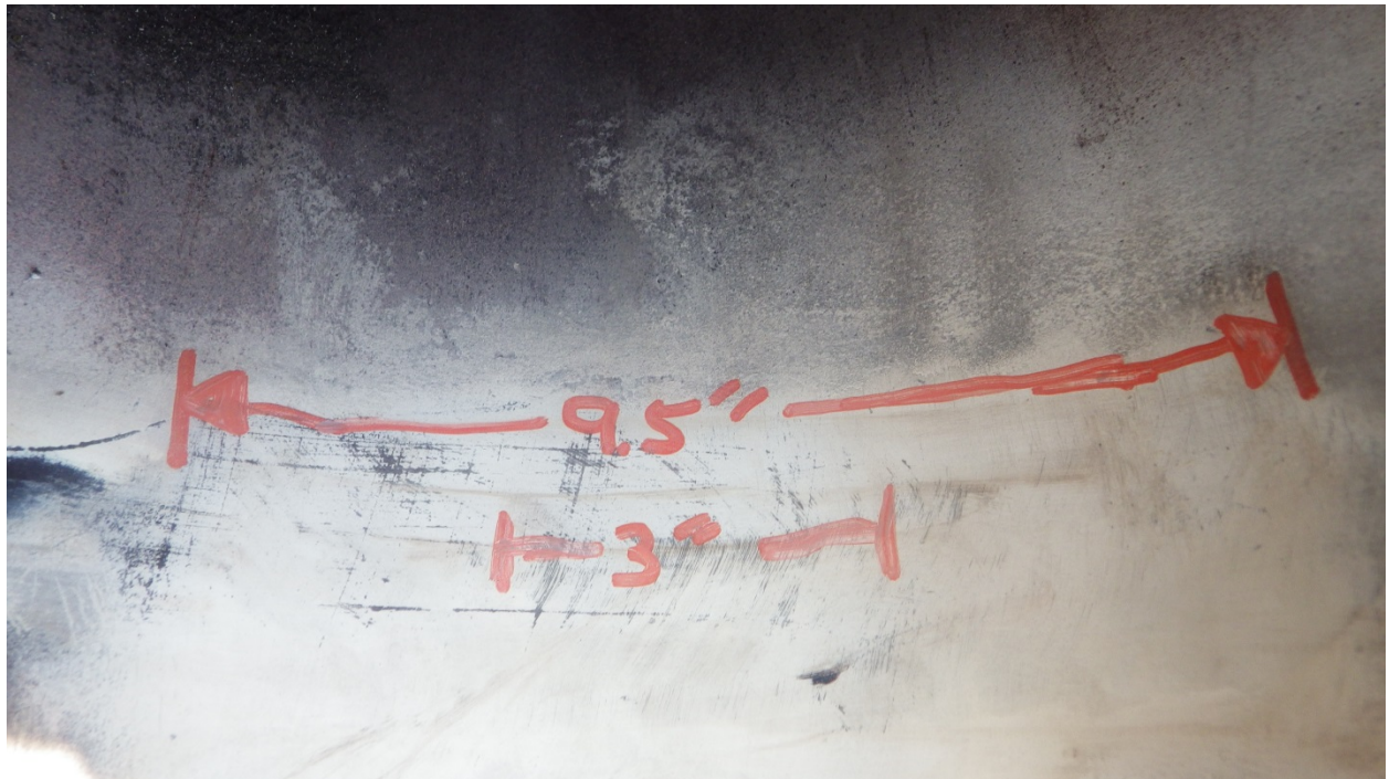
Burner side – outer partial crack
