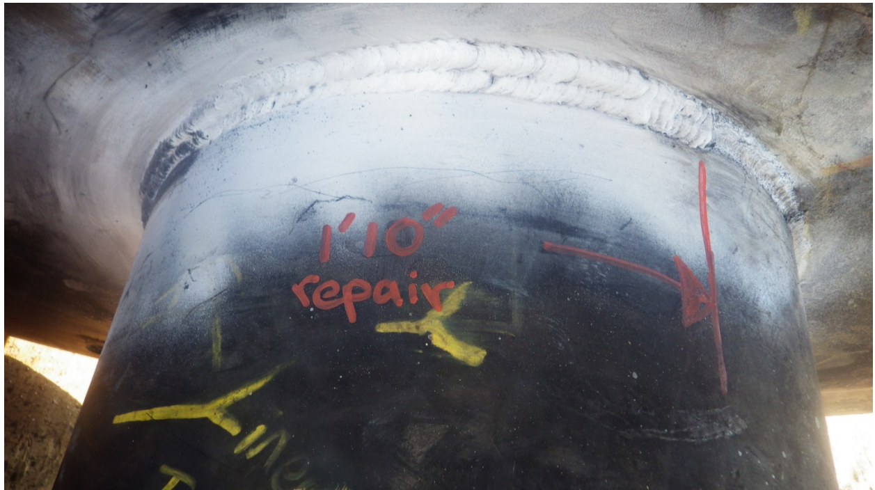
Burner side – outer partial crack
