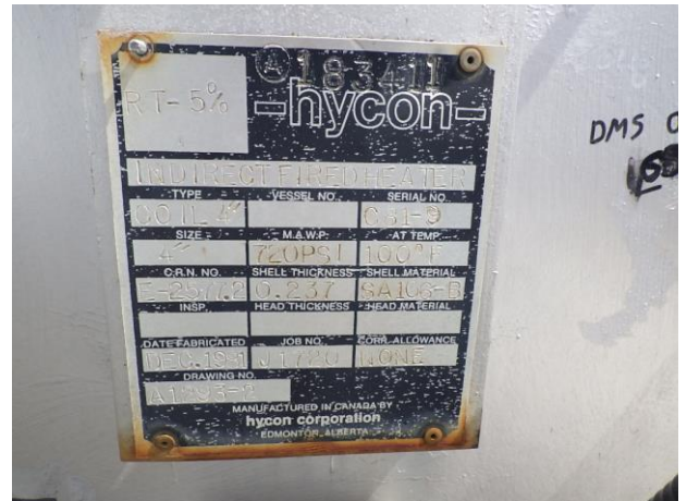
VESSEL DATA PLATE
