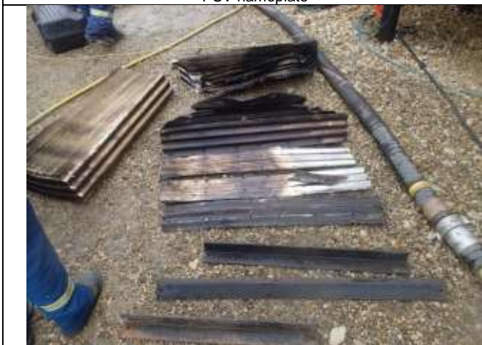
May 2017 Internal – Remainder of the vein pack removed from the vessel. No damage to the vessel shell or internal components
