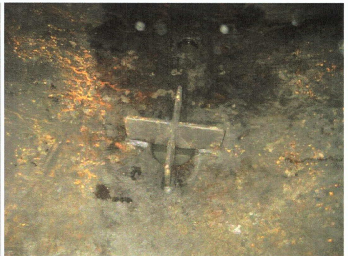
INLET DEFLECTOR AND VORTEX BREAKER
