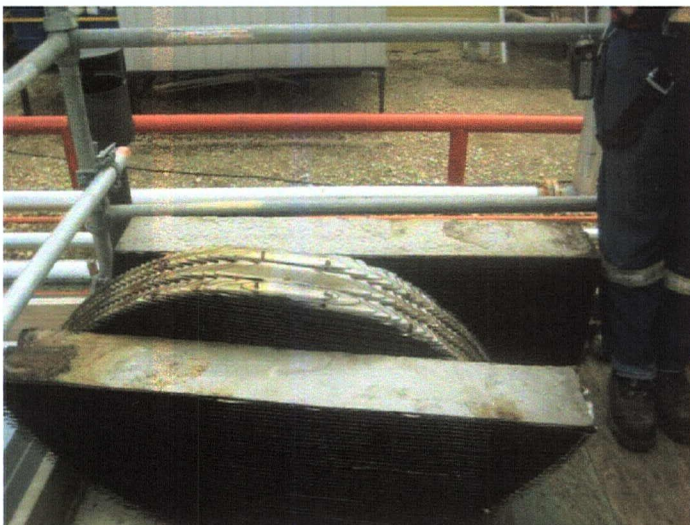
CHEVRON VANE PACK AS REMOVED
