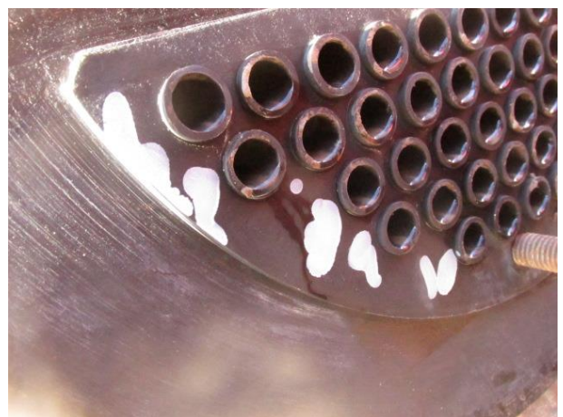
Tube sheet – 5 tubes marked for plugging after Eddy Current testing
