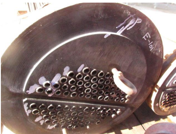
Tube sheet – 5 tubes marked for plugging after Eddy Current testing
