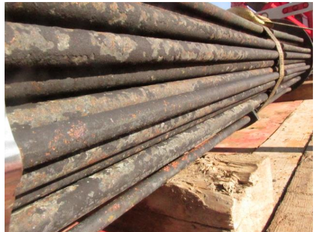
Tubes – scaly buildup
