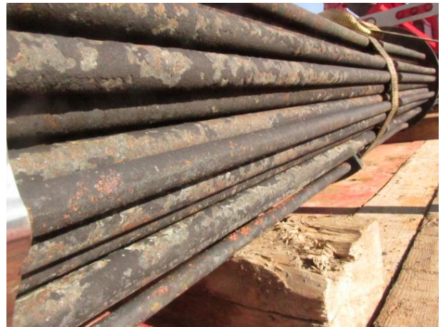
Tubes – scaly buildup
