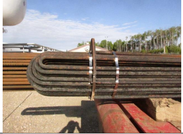
Tube bundle return bends – bundle tubes have insulation banding holding it together
