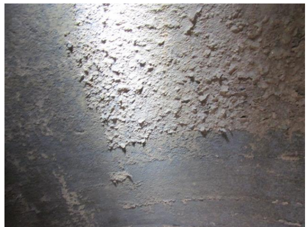
Bottom shell, scale and debris easily wire brushed clean
