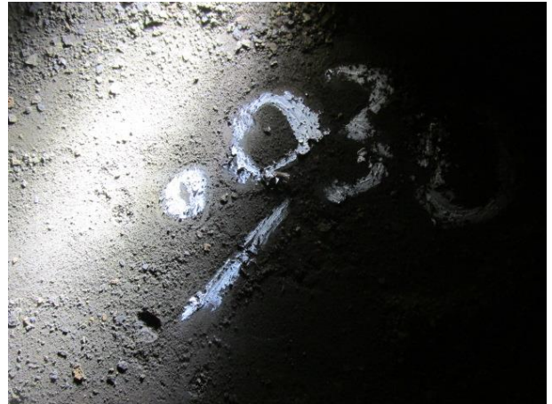
Corrosion on bottom head 0.030" deep
