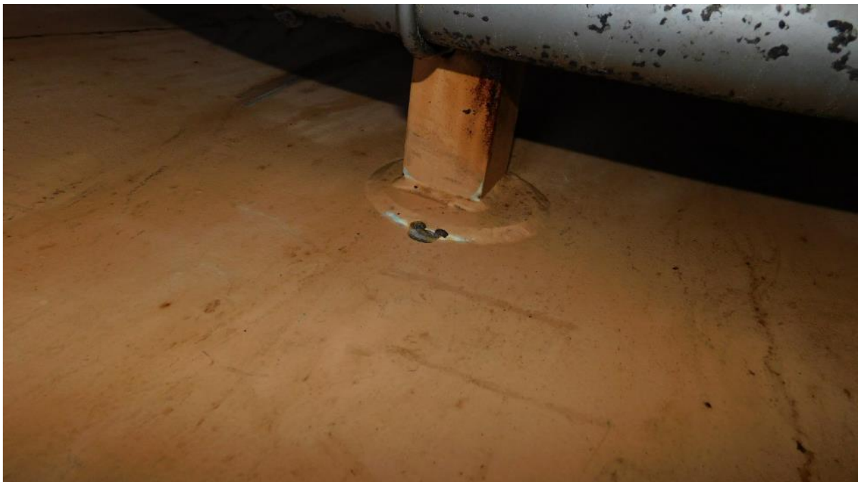
Photograph 13: Coating Failure on Pipe Support Reinforcing Pad
