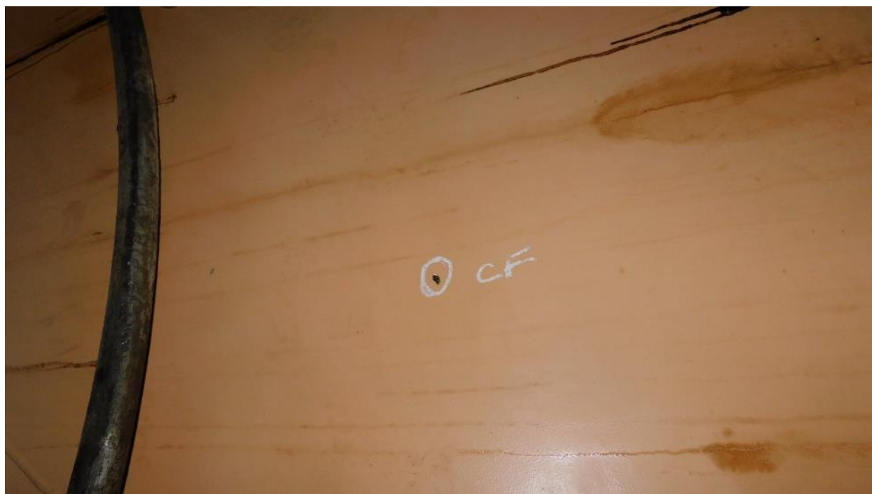
Photograph 14: Coating Failure on Bottom Plate
