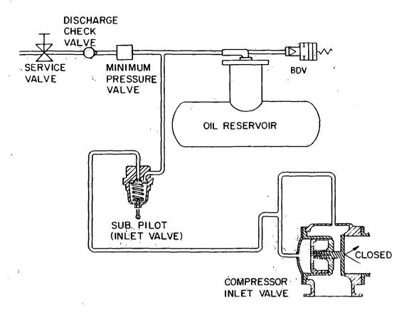
FIGURE 5-3 - FLOW DIAGRAM
