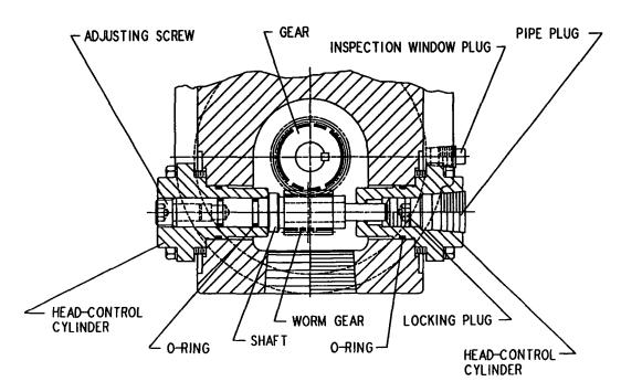
FIGURE 4-2 - MANUAL TURN VALVE ACTUATOR
