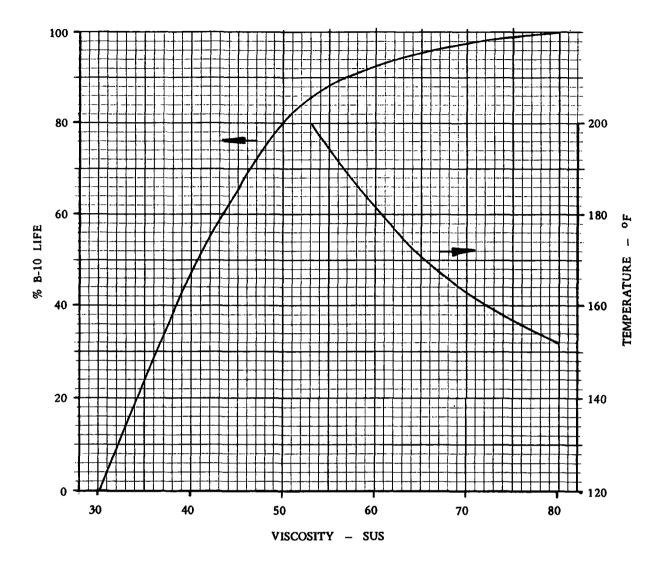
FIGURE 1-4 - EFFECT OF VISCOSITY ON B-10 LIFE
