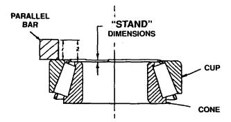
FIGURE 10-1 - BEARING "STAND" MEASUREMENT
