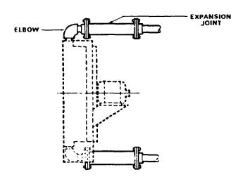
PIPING SCHEMATIC OF COOLER WITH FLANGED CONNECTIONS.
