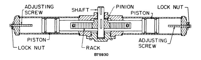
FIGURE 4-1 - AUTOMATIC TURN VALVE ACTUATOR
