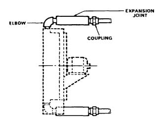
PIPING SCHEMATIC OF COOLER WITH SCREWED CONNECTIONS.
