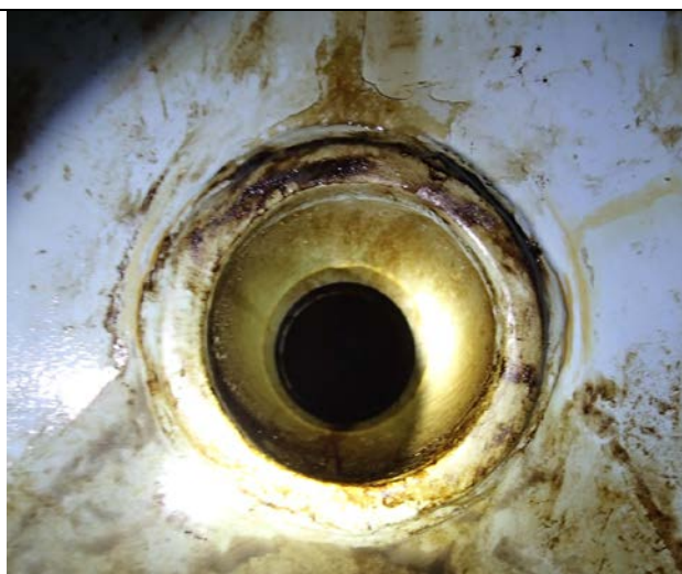
The desand outlet nozzle at the bottom of the vessel.
