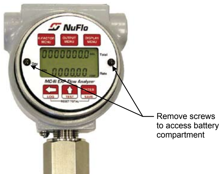
Figure 6.3—Removal of faceplate/keypad assembly
