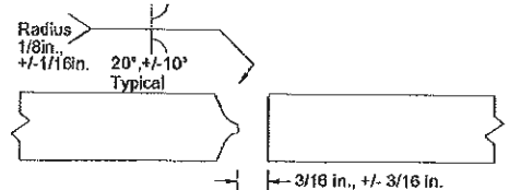
Figure 12 Double J Butt
