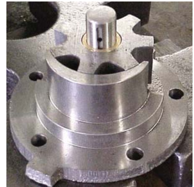
Figure 5, Pressing the idler pin
