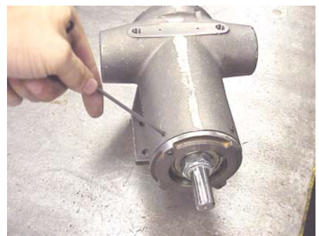
Figure 24, Tightening cone point setscrew
