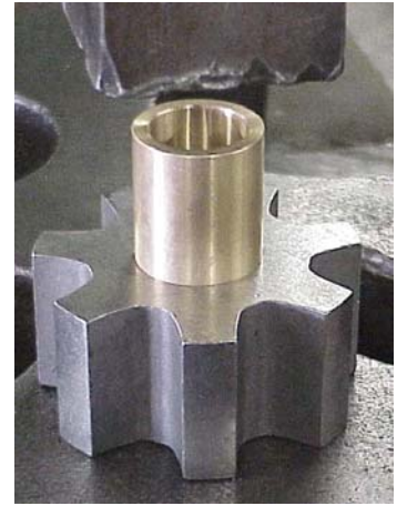
Figure 4, Pressing idler bushing
