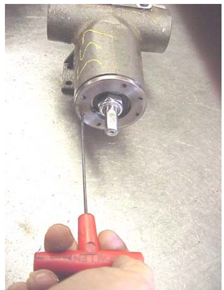
Figure 25, Tightening cup point setscrew
