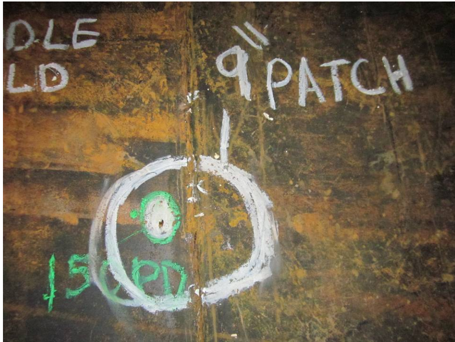
Photograph #18: 9 inch Round Recommended Patch
