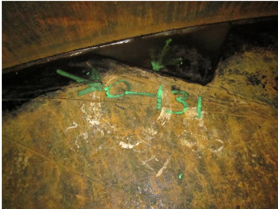
Photograph #16:MFL Indication | Minimum UT 0.131 inch
