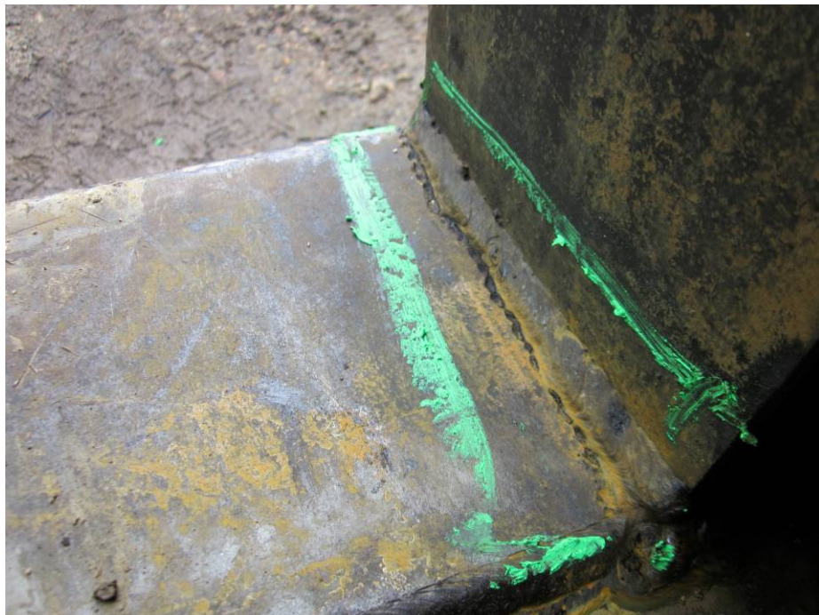
Photograph #41: Corrosion on Manway Weld
