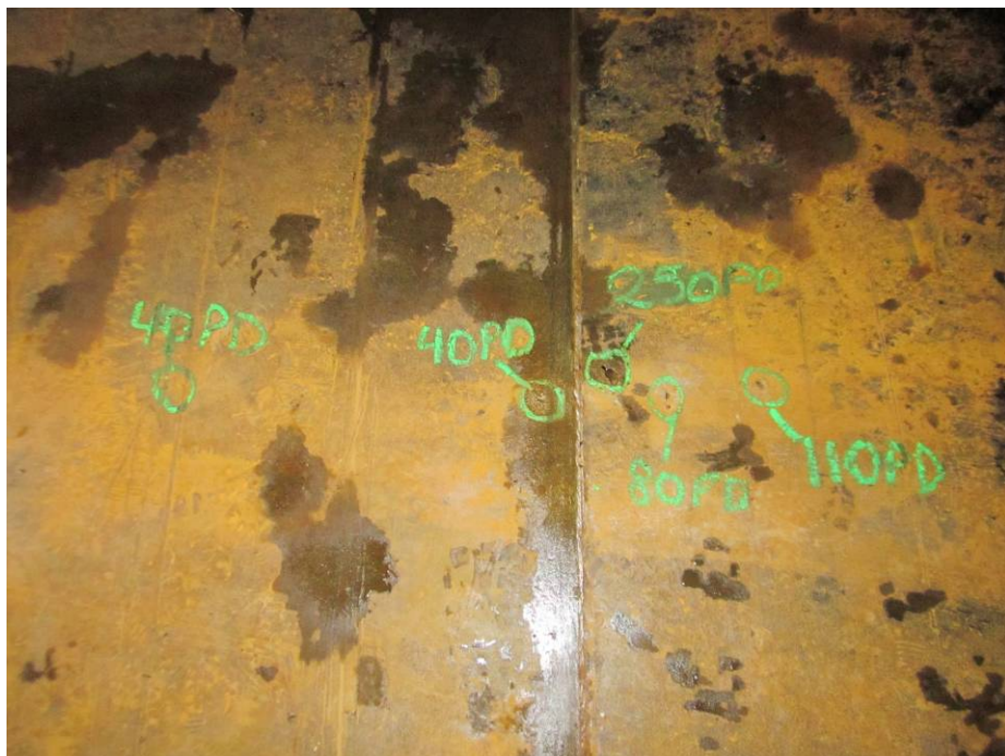
Photograph #11: Topside Pitting (Suspect Mechanical Damage)
