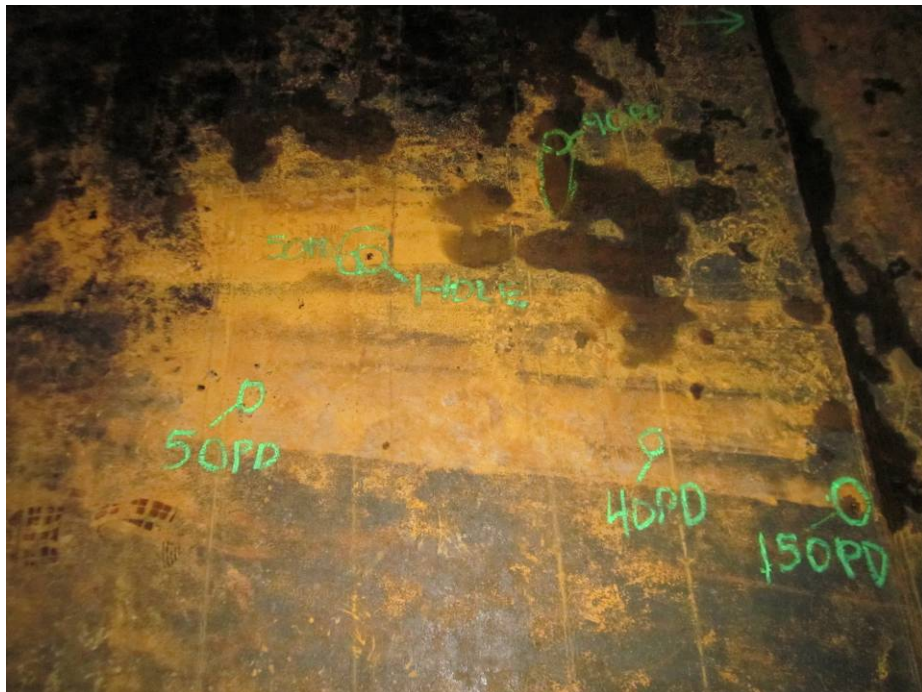
Photograph #13: Topside Pitting (Suspect Mechanical Damage)
