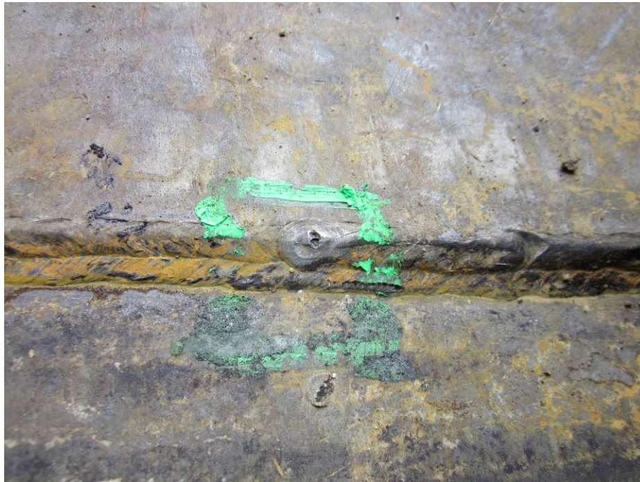
Photograph #40: Pinhole on Manway Weld
