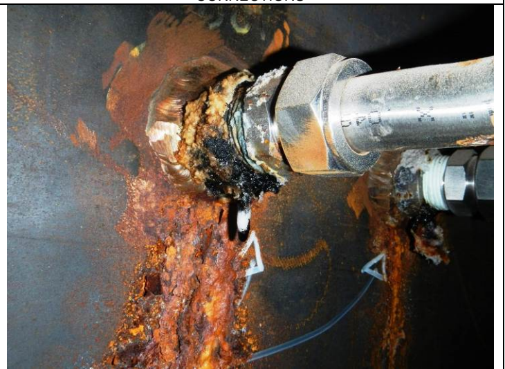
SIGNS OF LEAKAGE FROM THE TEST TAPS THREADED CONNECTIONS
