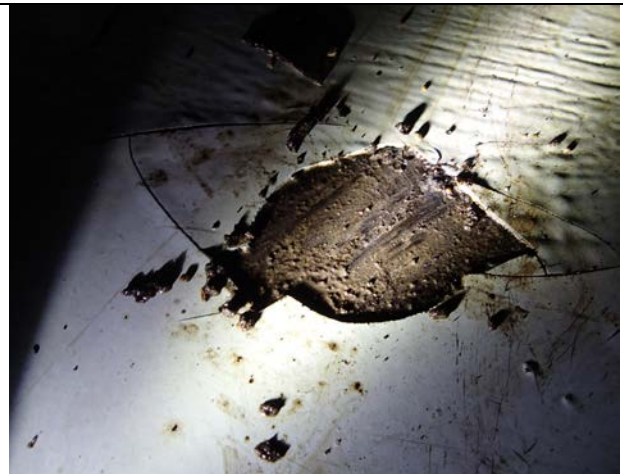
Area of coating failure in the bottom of the vessel from the firetube end to the sales end of the vessel. Coating was applied too heavily.
