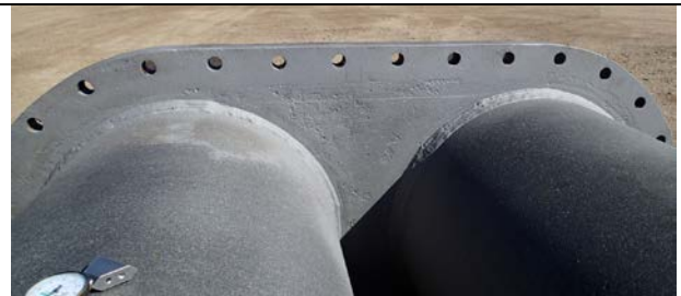
Tube sheet minor corrosion occurring.
