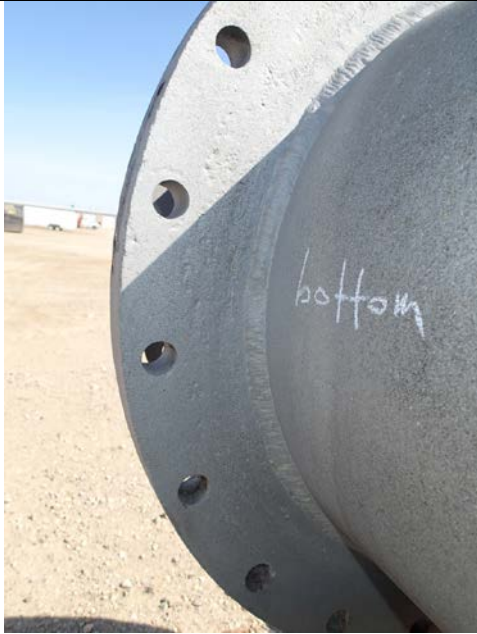
Bottom of the tube sheet on the north tube.
