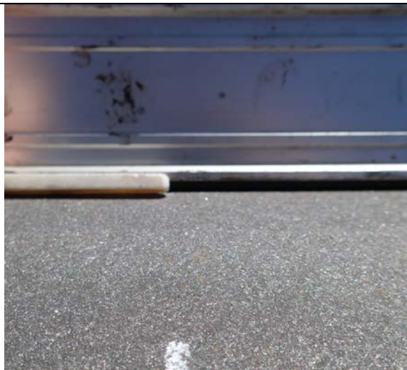
Close up of deflection on hot side.
