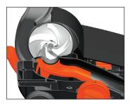
Efficient Impeller Technology – A 17,000 rpm impeller is driven by a toothed belt. A separate toothed belt drives the brush at approximately 3,000 rpm. This system makes the most efficient use of the motor power for powerful suction and brush action.
